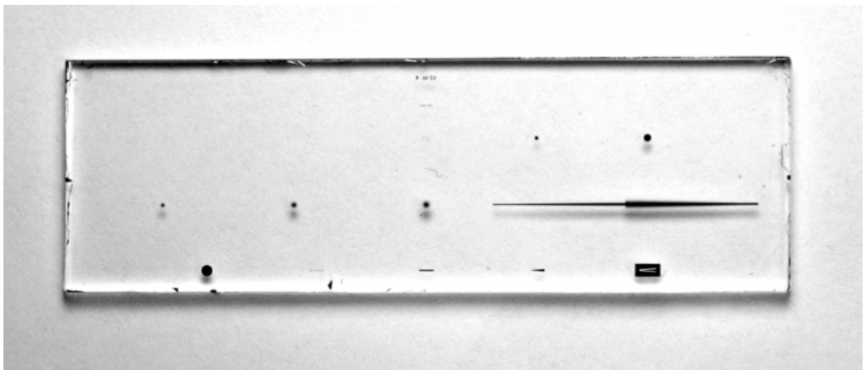
Fig. 1. A test sample for the NIRCam coronagraphs (Krist et al., 2006).
